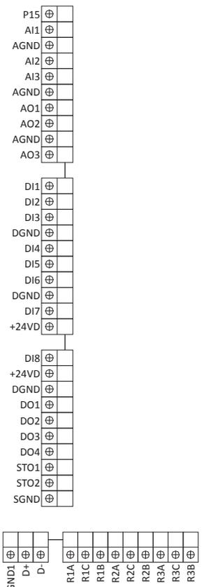
AGND, DGND & GND1 are internally isolated.
